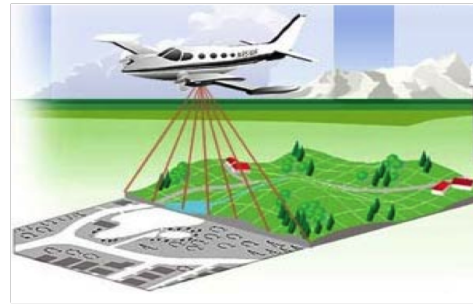
Figure 2: Airborne laser scanning technique
