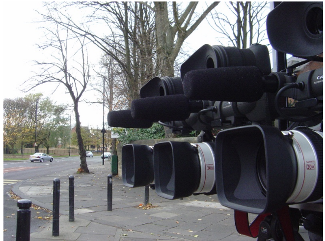
Fig. 2 Camera configuration used to capture footage for immersive video (used with permission).
