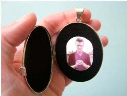
Close up of 'Locket' (Figure 2) digital jewelry piece made from silver, velvet, digital screen, memory card, rechargeable battery, electronic components. Once opened an image is displayed. The piece can be customized to show one image or a succession of images on repeated opening of the locket.
