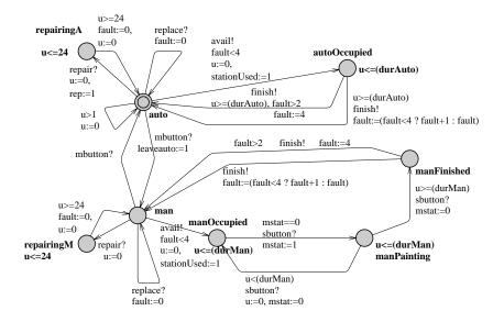
*Figure 3.* The paint station (Key: u: clock, fault: fault severity, mbutton: toggle manual/automatic painting, sbutton: press/release manual paint button, mstat: global flag denoting that manual painting is in progress, leaveauto: decoration that flags a mode change to manual mode).
