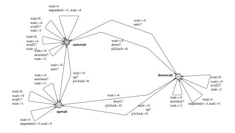
*Figure 4.* Boxes waiting to be channelled to the appropriate station (Key: wait: dispatched items waiting in queuing area, unpainted: overflow queue ot items failing to reach paint station, plclock, p2clock: local clocks of paint stations).
