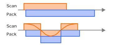
*Fig. 2.* Fixed (top) and flexible (bottom) scheduling, involving function postponement. Curved line represents value of scanning function
