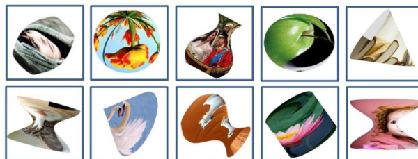
Figure 1: PiSHi asks the user to click on the upright orientation of 10 distorted pictures. Eight of these pictures are for evaluating the user, and have different hardness rates to be clicked correctly. The other two pictures are under observation of multiple users to be chosen in order to update the captcha database.
